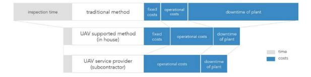
In the traditional method you have to shut down the plant, get an inspector to the location, prepare your gear, start roping down, perform a visual inspection, rope up, turn the turbine and start the roping process again and
